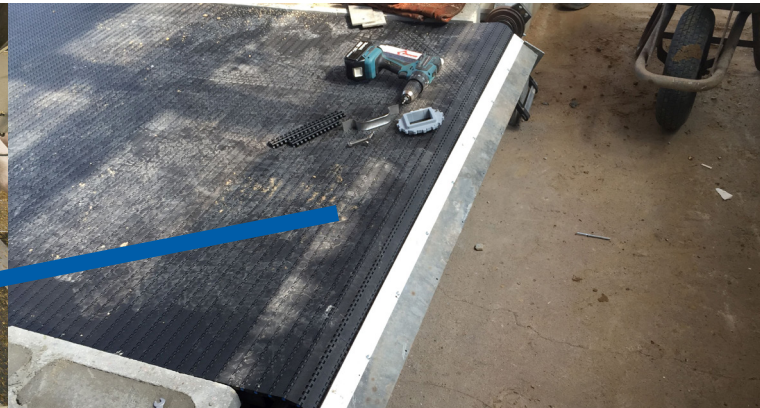
Investigation of the novel emission reduction measure „pig toilet“ in the KfreePig project: A porous, circumferential belt (right picture) is integrated in the defecation area. It ensures early separation of feces and urine and ensures that the animals use separate feces and lying areas (photos: Ralf Remmert).
